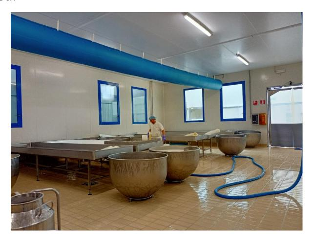
In the CAULDRON ROOM the cheesemakers add the **rennet**, **yeast** and penicillum roqueforti to the pasteurized milk in each cauldron, and they carefully control the coagulation and curding process, a combination of turning and resting, performed with the help of two tools – the harp, which is used to move the milk, and the flags, which are used to stop the circular movement of the milk.
